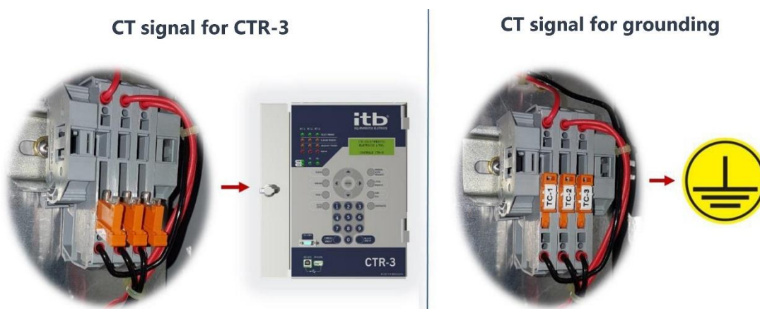
Figure 7: Procedure to short circuit the CTs.
